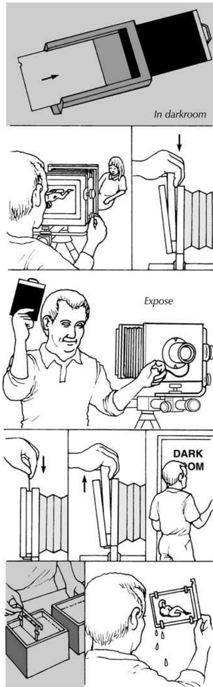
Figure L.4 How a picture is exposed with a 4 × 5 in camera, using a sheet film holder.
